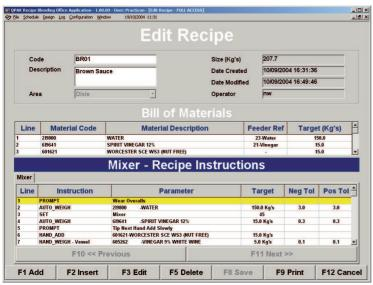
Weighment details are shown sequentially together with the Net Weight readings and Bar Graph indications representing the difference between the Actual Weights and the Target Weights. The Bar Graph positions and colours indicate the actions required from the operator.
