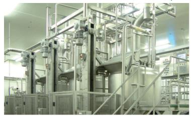
Batches are produced by weighing, mixing and cooking ingredients in a number of identical heated weigh-mix vessels.
