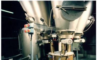
A number of weigh-mixers including portable mixing bowl 'Collet' type are fitted with shop floor terminals as are a number of hand-weigh stations in the prep area.
