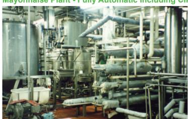
Mixing vessels fed from common ingredient weighers produce a continuous supply of product to milling and packing lines.
