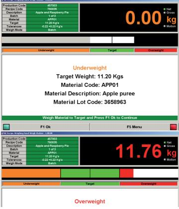
The system can prompt for ingredient lot/batch code numbers to be entered or scanned in via a barcode scanner for maximum material traceability.
